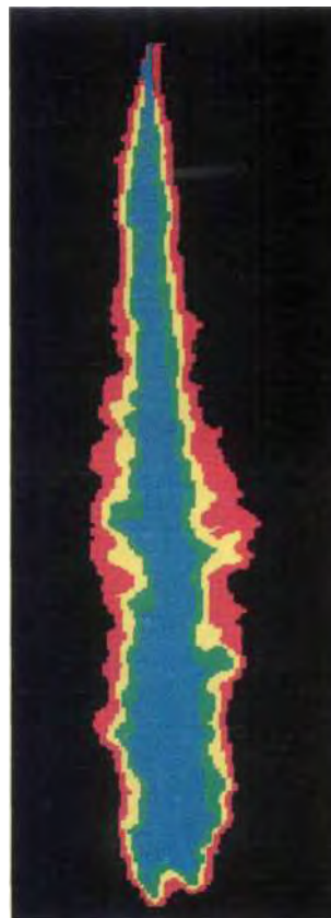
Electronic evaluation of an injection jet with diesel injection nozzles
