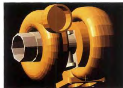
A surface model of a turbocharger, created with the aid of Computer Aided Design (CAD)
