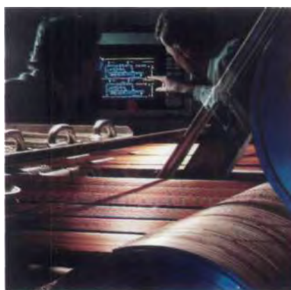
Computer-aided process control unit for a wire painting system
