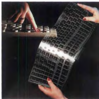
Multilayer-type foil switches with printed condensers
