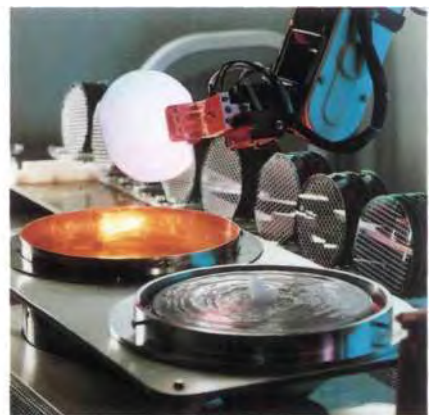
Fully automatic glass passivation with clean-room robots
