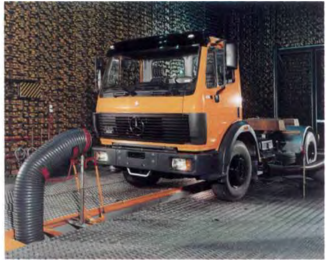
A truck made in our Wörth plant on the dynamometer for noise testing. An important measure on the way to further reducing the noise emissions of our trucks
