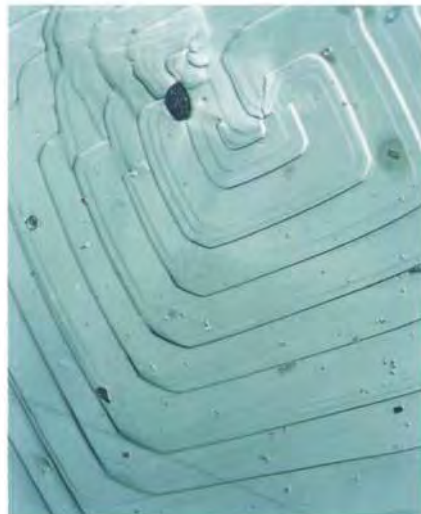
Growth shapes observed in the case of single crystals in high-temperature superconductors: part of research into anisotropic material properties
