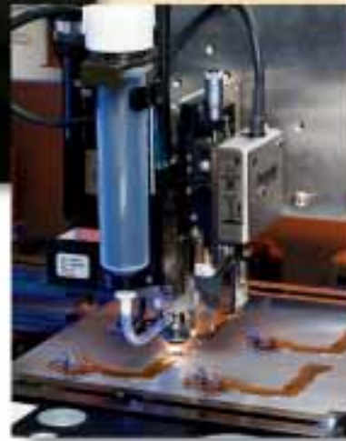
The Axiom™ X-1020 uses jetting technology to apply underfill to flip chips used on flexible printed circuit boards, such as those used in computer hard disk drives.
