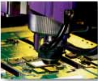
The Axiom™ X-1020 uses jetting technology to apply underfill to flip chips used on flexible printed circuit boards, such as those used in computer hard disk drives.
