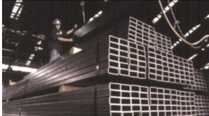
Each size and length of tubing is bundled for easy handling prior to shipment.
