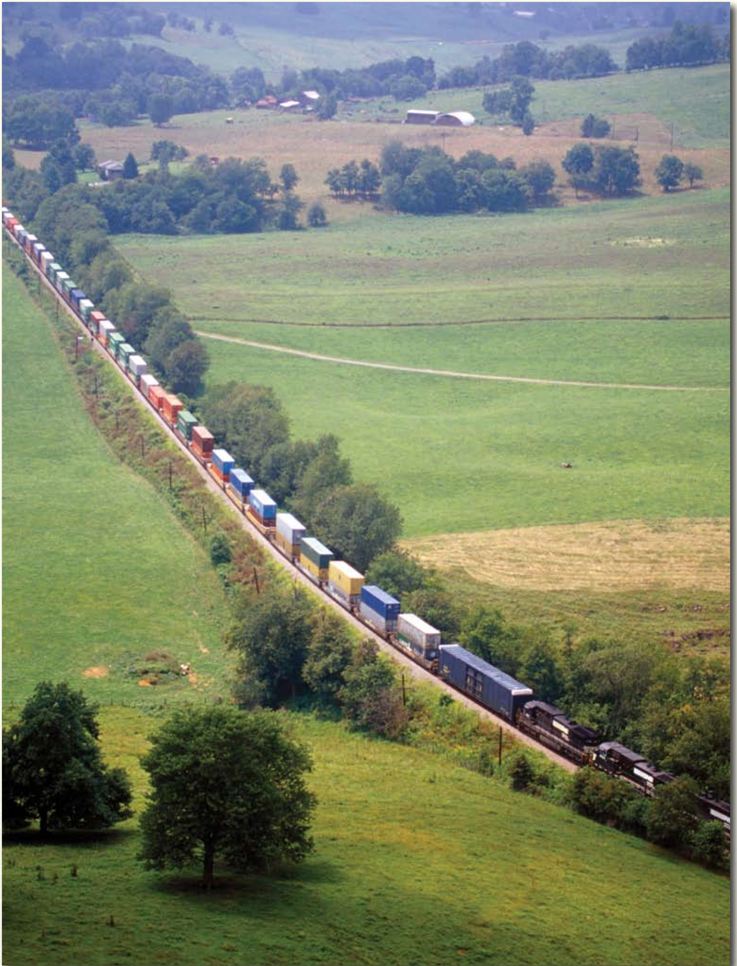
An intermodal train hauling mostly double-stacked containers moves northbound through the Virginia countryside near Interstate Highway 81.
