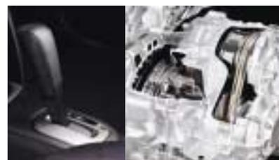
Continuously Variable Transmission (CVT)
