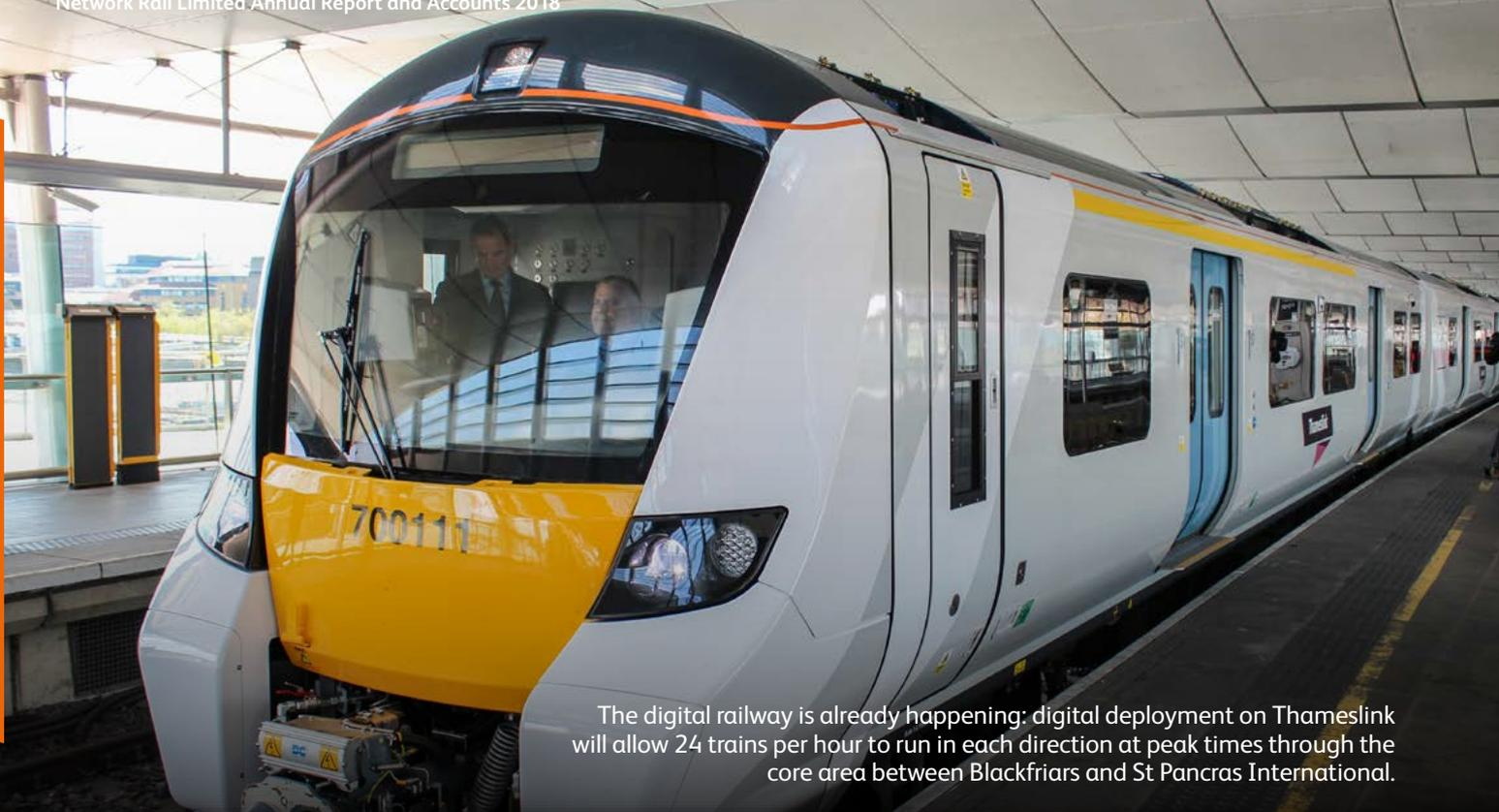
The digital railway is already happening: digital deployment on Thameslink will allow 24 trains per hour to run in each direction at peak times through the core area between Blackfriars and St Pancras International.
