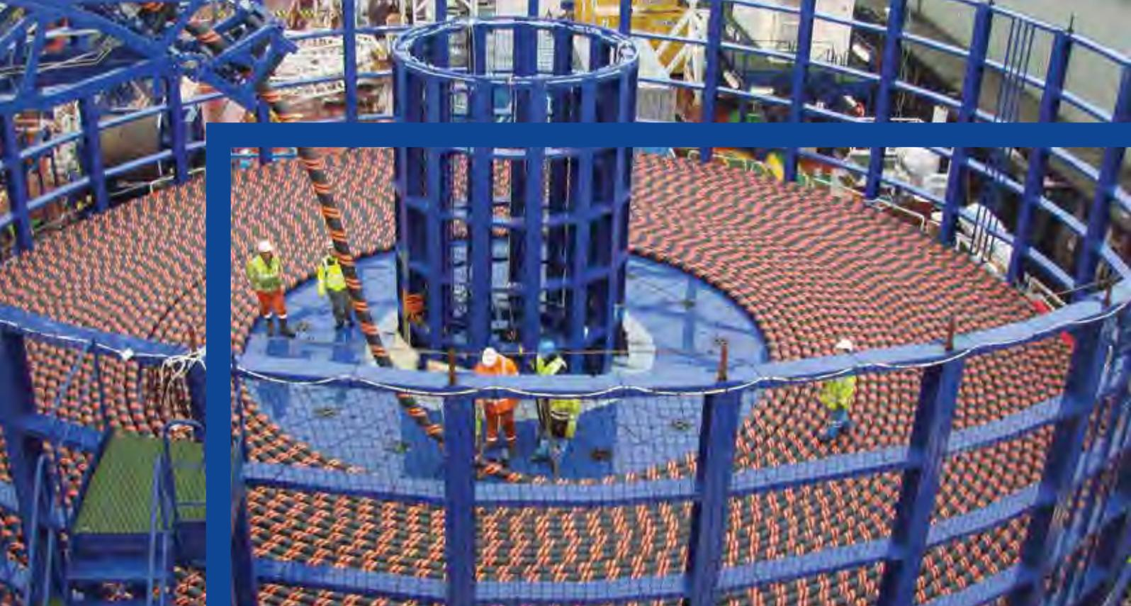
At the cable factory in Cologne, submarine cables weighing many tonnes can be stored on a turntable before shipment to customers
