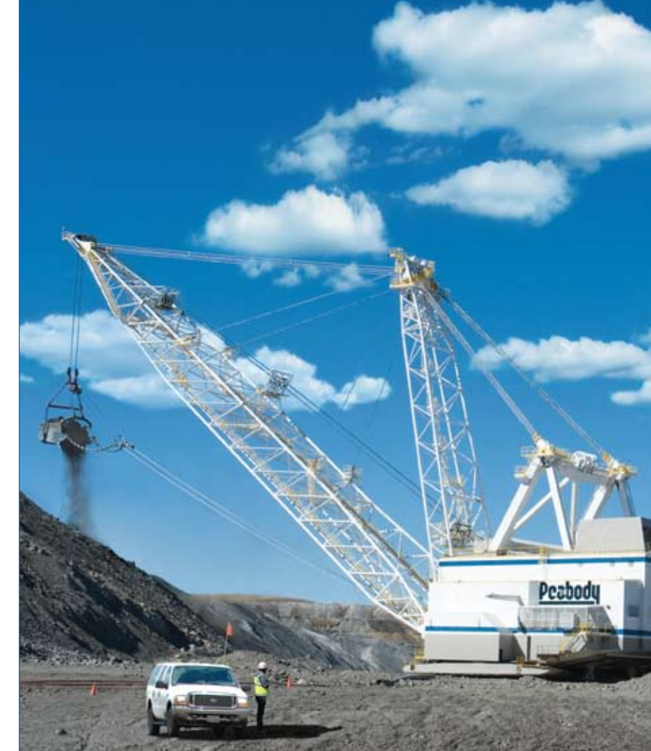
A new state-of-the-art dragline is increasing productivity and improving costs at Peabody's North Antelope Rochelle Mine, the nation's premier ultra-low sulfur mine.
