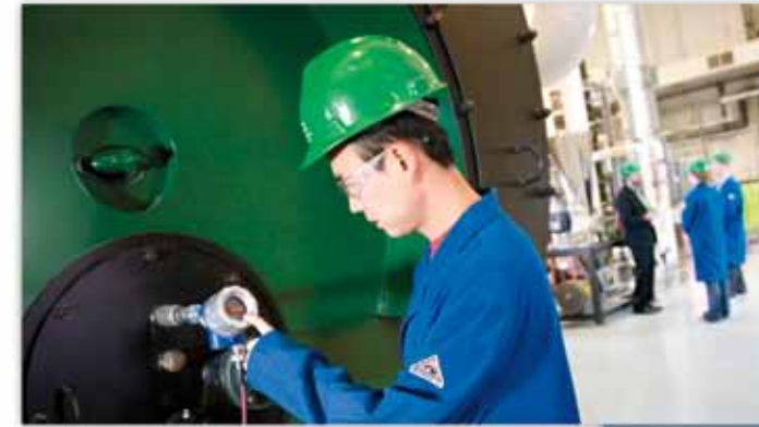
(Above) At Washington University in St. Louis, a researcher observes the boiler temperature as part of an oxyfuel demonstration for the Consortium for Clean Coal Utilization. (Right) Phase one construction at the GreenGen power project and carbon research facility in Tianjin, China, is nearing completion, with the first gasification unit expected on line in 2011.
