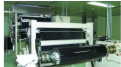
*Four different types of SPD-Smart light-control film are now being produced at the SPD Inc. factory in Incheon, Korea.*
