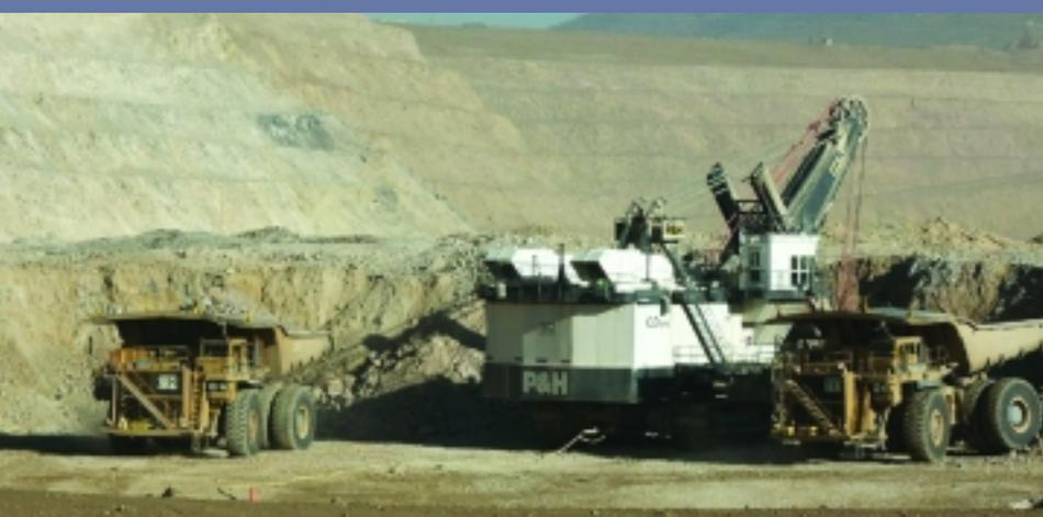
**Electric shovel loading 240-ton trucks at the Pipeline Mining Complex.**
