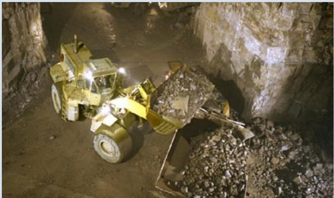
LOADING ORE WITH A FRONT-END LOADER AT THE TROY MINE.
