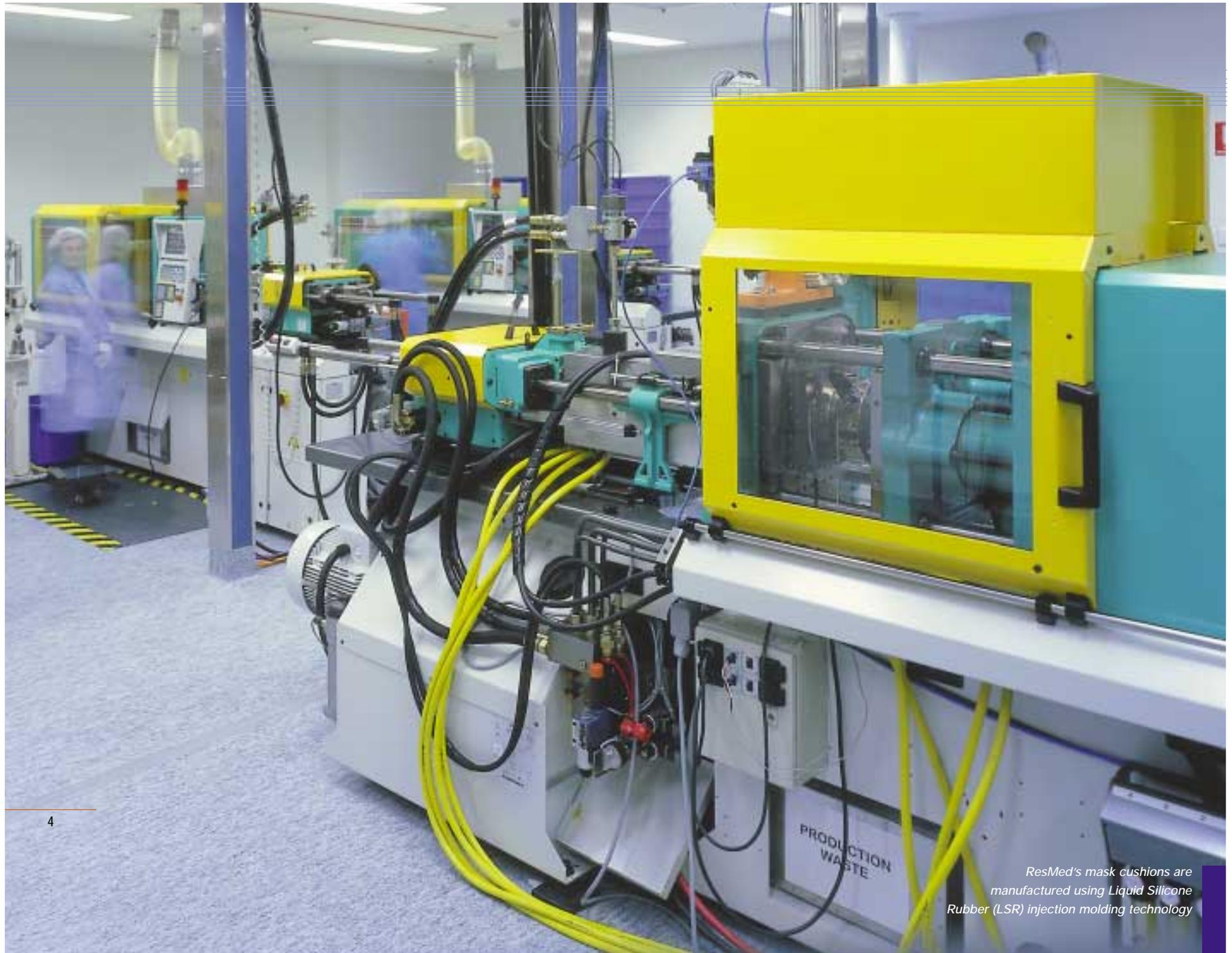
*ResMed's mask cushions are manufactured using Liquid Silicone Rubber (LSR) injection molding technology*
