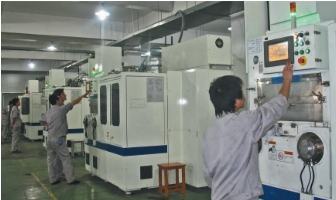
1 Installed monocrystalline furnaces.
