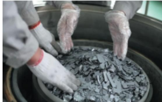
*Scrap polysilicon is loaded into a monocrystalline furnace.*
