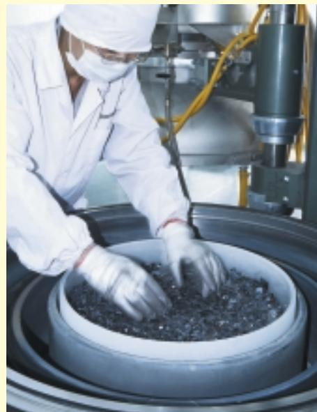
*Loading a crucible with feedstock*
