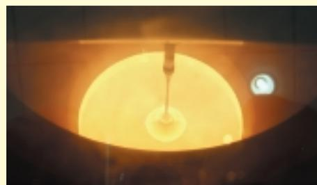
*Molten polysilicon inside a monocrystalline furnace*
