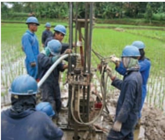
Figure 3: Portable compressor rig drilling a seismic shot-hole.
