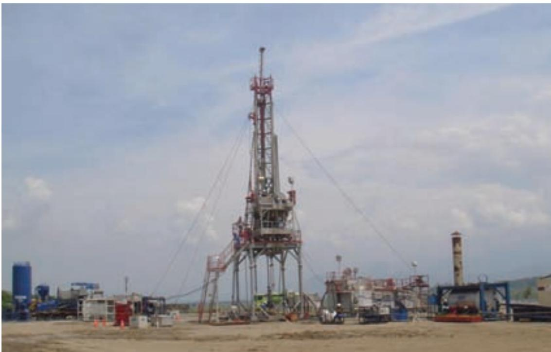
Figure 1: Lekom Maras HWO rig and surface equipment setting up for DST 3 on Pasundan-1 in November 2008.
