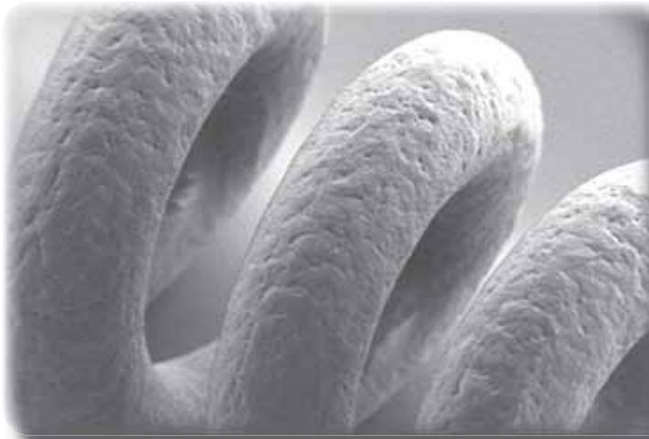
**Above:** Scanning electron microscopic image of an I-vation intravitreal implant coated with a SurModics drug-eluting polymer matrix. The coating is uniform and exhibits no cracking or peeling away from the surface.
