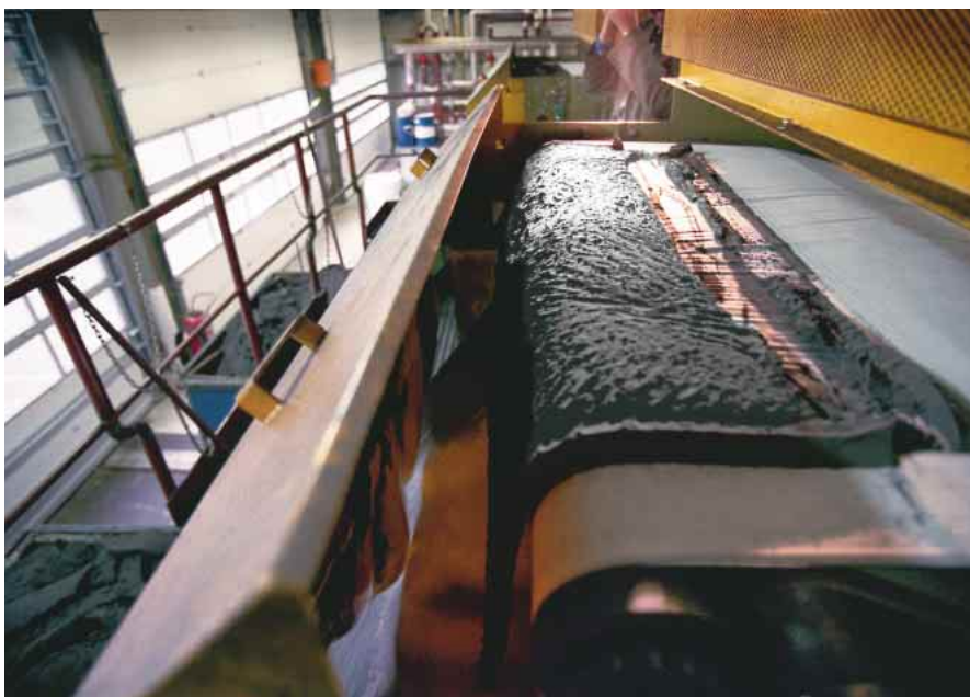
Filter beds at SKF Österreich in Steyr separate grinding waste from coolant liquid so that both can be recycled.
