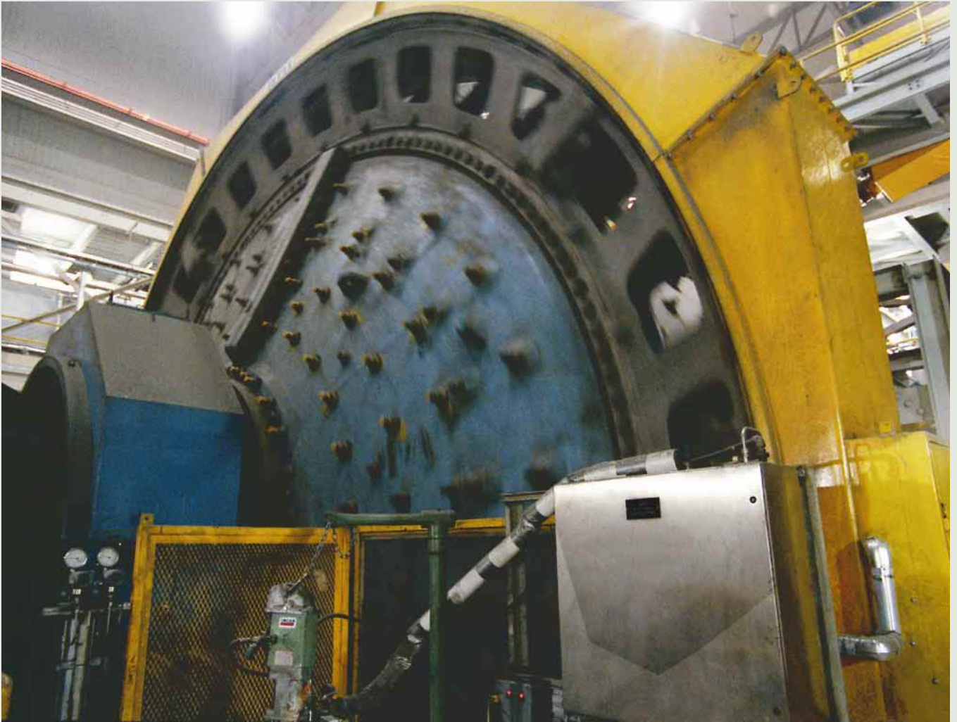
This giant grinding mill at Noranda Inc., Brunswick Mine, in eastern Canada, is equipped with spherical roller bearings from SKF. The crushed zinc ore is delivered directly from the mine and is ground into smaller particles in the mill before going to the flotation process.
