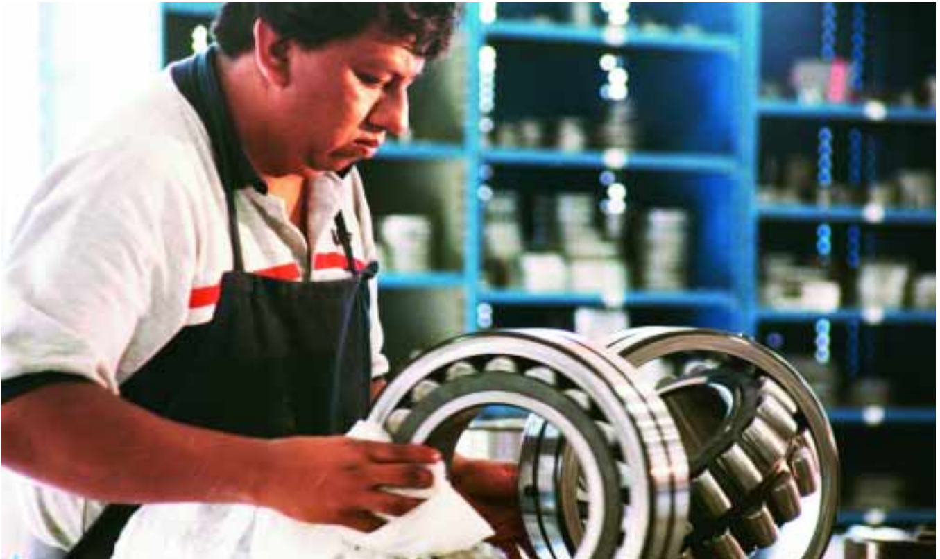
Rodolfo Cruz-Gutierrez inserting Solid Oil (lubricant) in spherical roller bearings at the SKF plant in Puebla, Mexico.
