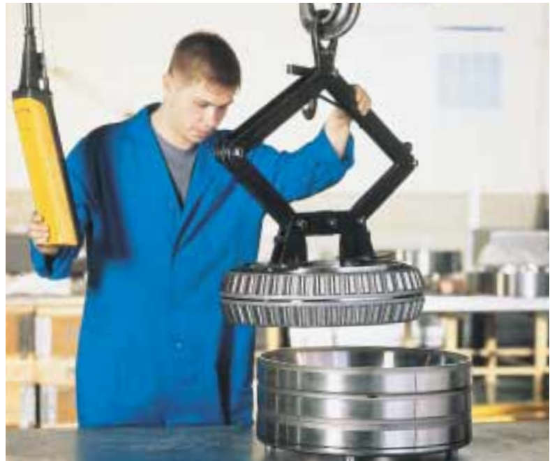
Assembly of four-row taper roller bearings, SKF GmbH, Schweinfurt, Germany.
