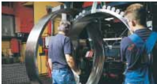
Assembly of large size bearings, SKF Sverige, Göteborg, Sweden.
