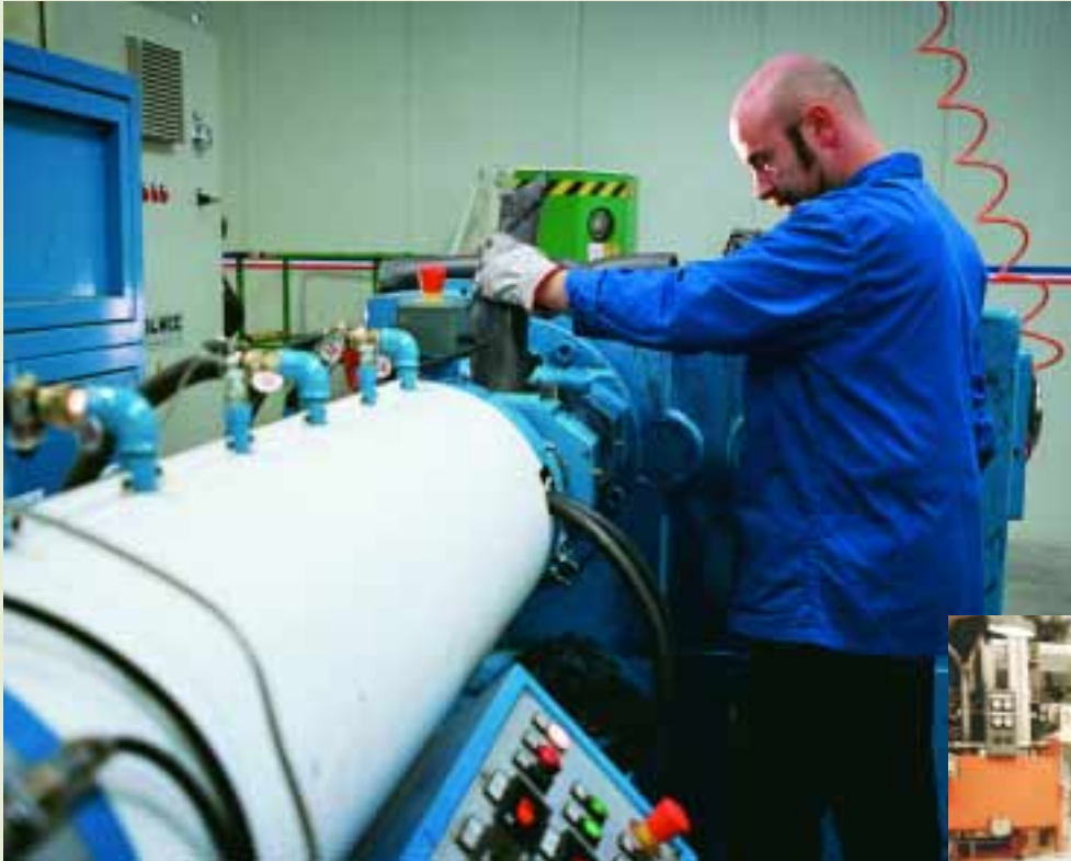
Rubber extruding machine at the RFT seals manufacturing plant at Varese, Italy.
