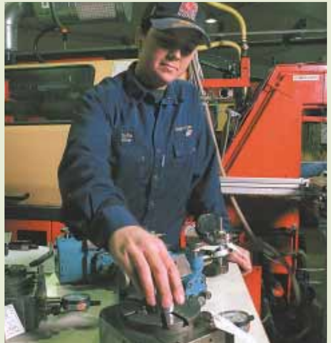
Drilling of lubrication holes in outer rings for spherical roller bearings and manual inspection of the dimensions of soft-machined bearing rings, Ovako Steel, Hofors, Sweden
