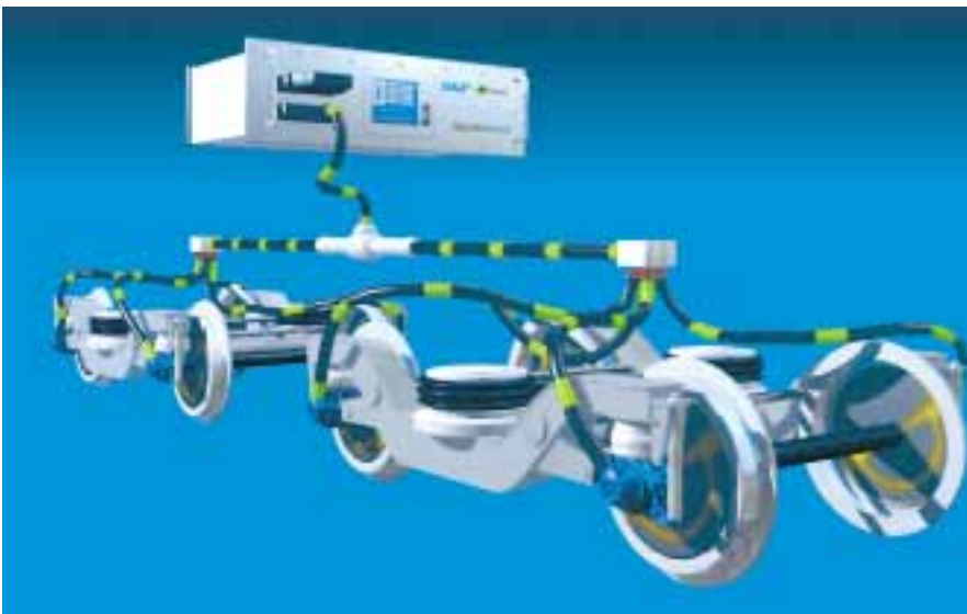
The highly sophisticated bogie-monitoring system (BoMo), jointly developed by SKF and Sécheron.
