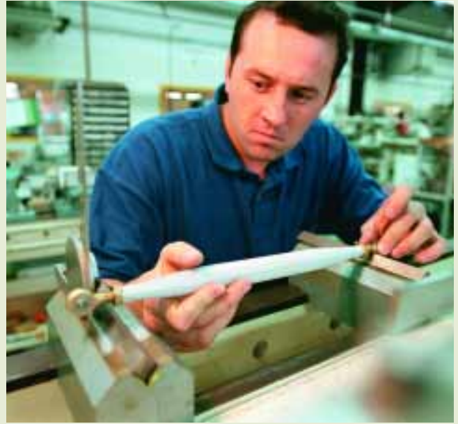
Final measuring and inspection of an airframe rod carried out by Canterro José at the SARMA plant in St. Vallier, France.
