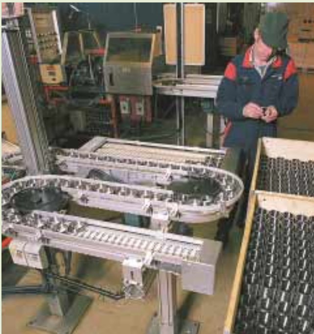
Drilling of lubrication holes in outer rings for spherical roller bearings and manual inspection of the dimensions of soft-machined bearing rings, Ovako Steel, Hofors, Sweden
