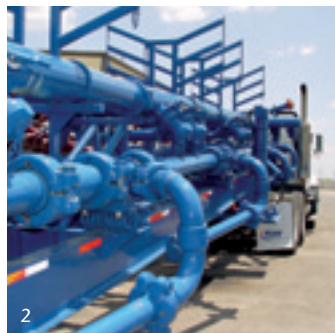
1. Pump in assembly at Weir Gabbioneta in Milan, Italy. 2. A safety iron manifold trailer unit at Weir SPM, Fort Worth. 3. Weir SPM's main workshop at Fort Worth, Texas.
