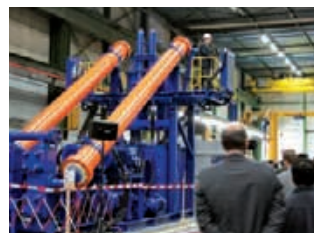
Part of Minerals de-watering range, the patented GEHO APEXS® power saving pump moves large volumes of abrasive, corrosive slurries at high pressures.
