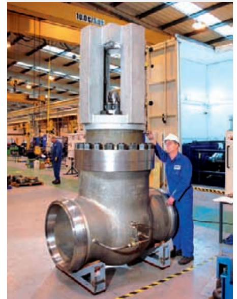
The five-metre Hopkinsons® Main Steam Isolation Valve
