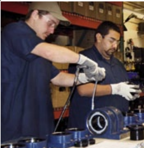
Tyler Klander, warehouse associate, and Juan Barajas, shipper/receiver, assemble spherical roller bearing steel-housed units at our newly acquired plant in Ferndale, Wash.
