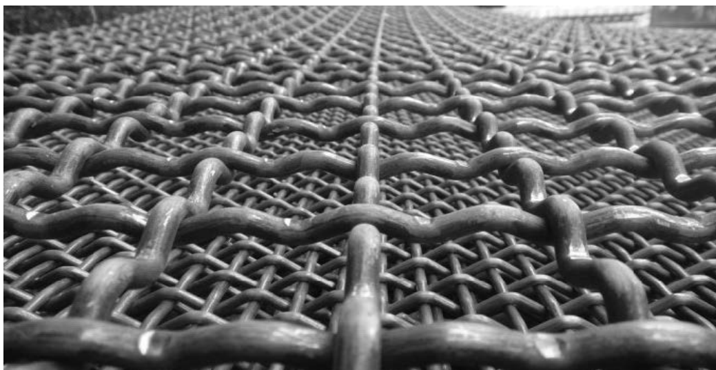
High Carbon, Bright Gravel Screen Wire (woven into an industrial screen)
