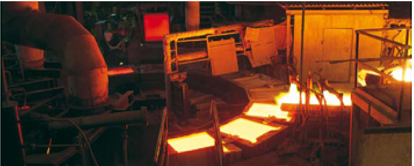
Anode casting at Tuticorin copper smelter, India
