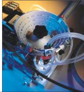
This automated equipment quality-tests surface-mount passive electronic components and inserts them into tape-and-reel packaging.
