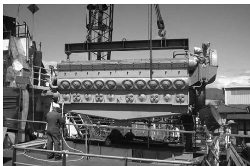
This 20-cylinder Electro-Motive Diesel engine delivers 5,000 horsepower to marine, power and industrial applications.
