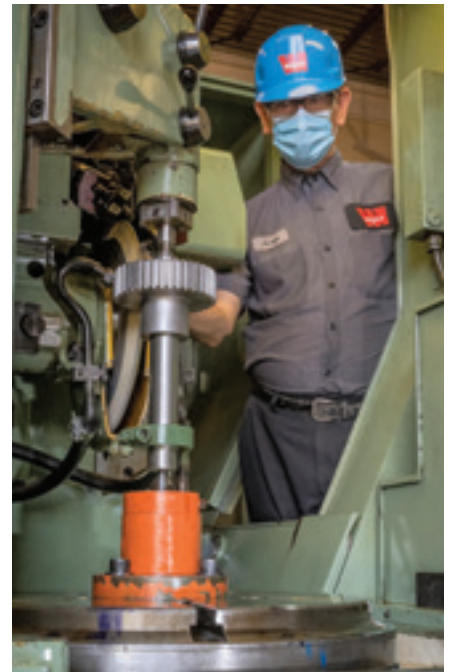
An ERS technician grinding straight tooth gear at the LaSalle branch.
