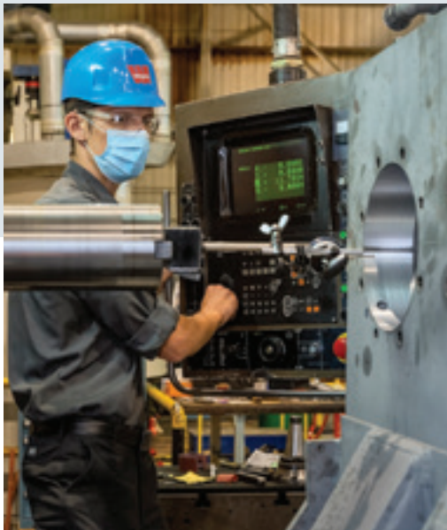
Engineered Repair Services Technician horizontally boring a bearing journal.
