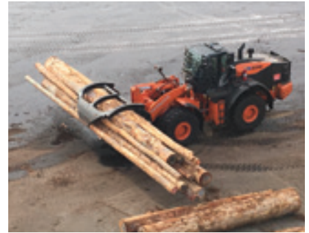
A Hitachi ZW370-5B Wheel Loader with log grapple working in the forestry industry on Vancouver Island.
