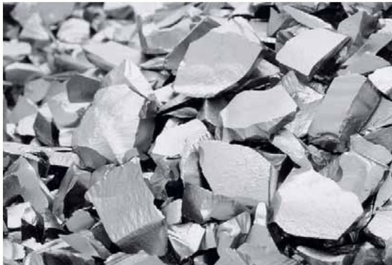
**Hyperpure polycrystalline silicon for semiconductor and photovoltaic applications.**
