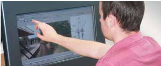
Zytronic's touch sensor technology is also readily scalable in size, allowing customers to use sensors ranging in size from 6 inches to 82 inches. Additional customisation can be provided, including printed borders, logos, etc.; non-rectangular shapes; shaped polished edges; and different glass substrate thicknesses from 1mm to 12mm.
